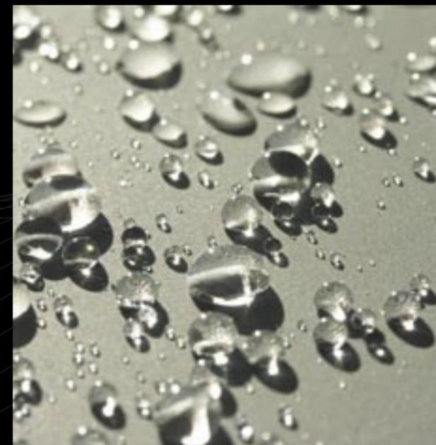
The Dinamic CCC cladding-elements are finished with a special hydrophobation process making the finished product resistant to water.
